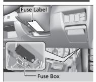
Fuse locations are shown on the label. Locate the fuse in question by the fuse number and label number.
