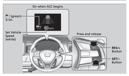
When driving at about 30 km/h or above: Take your foot off the pedal and press the RES/+ or SET/- button when you reach the desired speed. The moment you release the RES/+ or SET/- button, the set speed is fixed, and ACC with Low Speed Follow begins.
