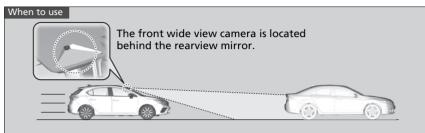
The system starts monitoring the roadway ahead when your vehicle speed is about 5 km/h or above and will search for a vehicle (including motorcycles), pedestrian, or moving bicycle in front of you.
