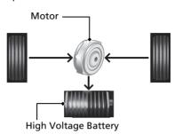
When decelerating without the accelerator being depressed or the brake pedal being applied, or while driving downhill, the electric motor acts as a generator that recovers a portion of the electrical energy that was used to accelerate the vehicle. This regenerative braking slows the vehicle in a manner similar to engine braking in a petrol-powered vehicle.
