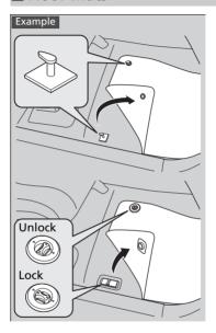
The driver's floor mat hooks over floor anchorages, which keep the mat from sliding forward.
