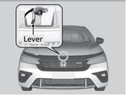
**3.** Pull up the bonnet latch lever (located under the front edge of the bonnet to the centre) and raise the bonnet. Once you have raised the bonnet slightly, you can release the lever.
