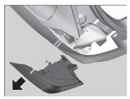
**3.** Pull the light assembly out of the rear pillar.
