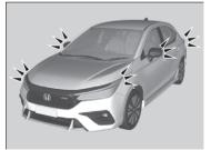
If the power system is turned on successfully, some exterior lights flash six times.
