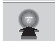
**3.** Without depressing the accelerator pedal, press the **POWER** button while depressing the brake pedal.
