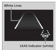
When the LKAS is suspended, green lines on the gauge change to white lines or disappear, and the beeper sounds (if activated).
