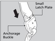
2. Line up the triangle marks on the small latch plate and anchorage buckle.
