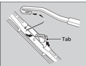
**2.** Press up on and hold the tab, then slide the holder off the wiper arm.
