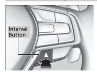
Press the Interval button to change the ACC with Low Speed Follow following-interval. Each time you press the button, the following-interval (the interval behind a vehicle detected ahead of you) setting cycles through extra long, long, middle, and short following-intervals.
