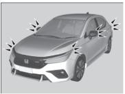
If the power system is turned off successfully, the exterior lights flash once.
