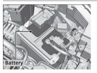
The condition of the battery is monitored by a sensor located on the negative terminal of the battery. If there is a problem with this sensor, the driver information interface will display a warning message. If this happens, have your vehicle inspected by a dealer.
