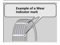
The groove where the wear indicator is located is about 1.6 mm shallower than elsewhere on the tyre. If the tread has worn so that the indicator is exposed, replace the tyre. Worn out tyres have poor traction on wet roads.
