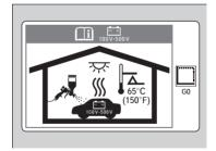
High temperature may damage the high voltage battery used to power the electric motor.
