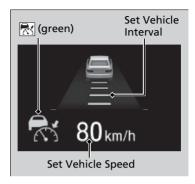
When ACC with Low Speed Follow starts operating, the vehicle icon, interval bars, and set speed appear on the gauge.
