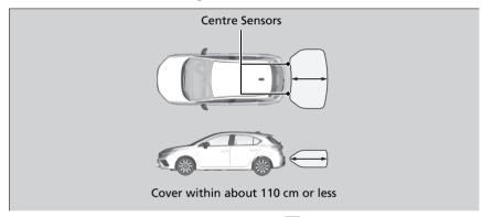
The system activates when the transmission is in  $\mathbb{R}$ , and the vehicle speed is less than 8 km/h.
