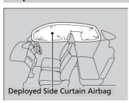
The side curtain airbag is designed to deploy in a moderate-to-severe side impact.
