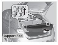
**3.** Disengage the support rods, then remove the luggage area cover.
