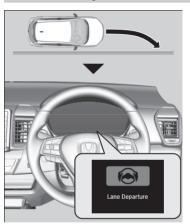
The front camera located behind the rearview mirror monitors left and right lane markings (in white or yellow). If your vehicle is getting too close to detected lane markings without a turn signal activated, the system, in addition to a visual alert, applies steering torque and alerts you with rapid vibrations on the steering wheel, to help you remain within the detected lane.
