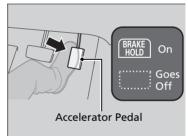
Depress the accelerator pedal while the transmission is in a position other than  $\boxed{\textbf{P}}$  or  $\boxed{\textbf{N}}$ . The system is cancelled and the vehicle starts to move.
