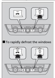
Press the wbutton to turn the air conditioning system on. Press the button (indicator off) to switch to the fresh air mode.
