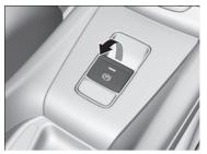
1. Make sure the parking brake is applied. The parking brake and brake system indicator comes on for 30 seconds when you pull up the electric parking brake switch.
