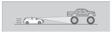
• When the camera cannot correctly identify the shape of the vehicle ahead of you.
