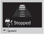
Your vehicle also stops, automatically. The **Stopped** message appears on the gauge. When the vehicle ahead of you starts again, if you press the **RES/+** or **SET/-** button, or depress the accelerator pedal, ACC with Low Speed Follow will operate again within the previously set speed.
