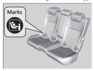
**1.** Locate the lower anchorages under the marks.
