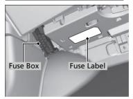
Fuse locations are shown on the label. Locate the fuse in question by the fuse number and label number.
