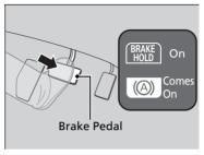
Depress the brake pedal to come to a complete stop. The transmission must not be in  $\boxed{\mathbf{P}}$  or  $\boxed{\mathbf{R}}$ .
