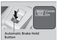
Fasten your seat belt properly, then turn on the power system. Press the automatic brake hold button.
