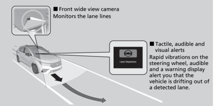
When you operate the turn signals to change lanes, the system is suspended, and resumes after the signals are off.
