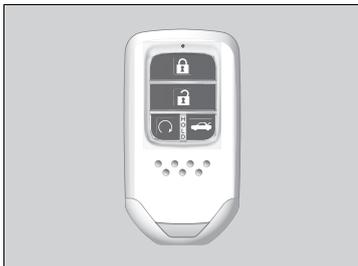
Use the key to turn on and off the power system, and lock and unlock all the doors and open the boot.
