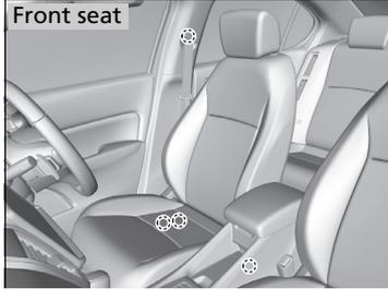
When replacing the seat belts, use the anchorage points shown in the images. The front seat has a lap/shoulder belt.
