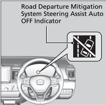
If the system operates several times without detecting driver response, the system beeps to alert you. After that, the Road Departure Mitigation System Steering Assist Auto OFF indicator comes on, the Road Departure Mitigation steering assist is temporarily stopped, and the system will only alert you with the warning sound.
