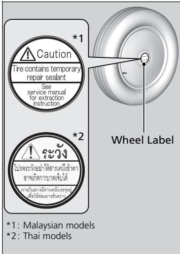
14. Apply the wheel label to the flat surface of the wheel.
