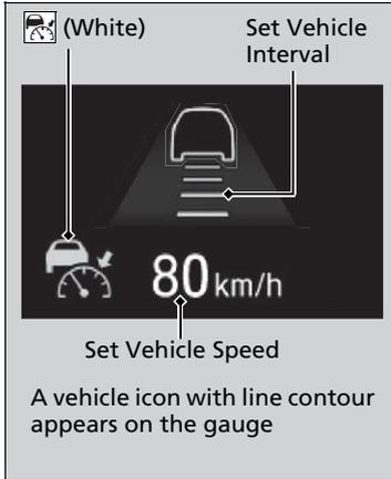
Your vehicle maintains the set speed without having to keep your foot on the brake or accelerator pedal.
