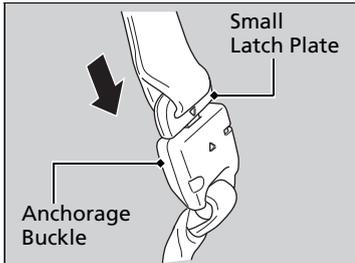
2. Line up the triangle marks on the small latch plate and anchorage buckle. Make sure the seat belt is not twisted. Attach the belt to the anchorage buckle.
