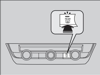
Press the rear demister button to demist the rear window when the power mode is in ON.
