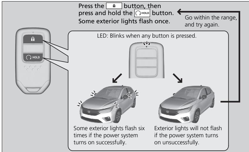
The power system is on for up to 10 minutes without you starting the vehicle. To extend the time for another 10 minutes during the first 10 minutes, press the **a** button, then press and hold the **HOLD** button.
