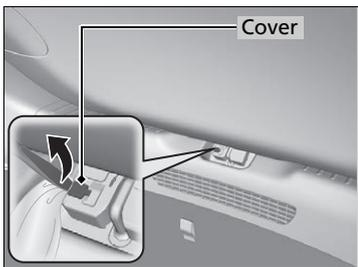
1. Use a flat-tip screwdriver and remove the cover on the back of the tailgate.
