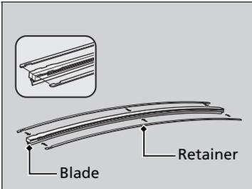
**4.** Remove the retainers from the wiper blade that has been removed, and mount to a new wiper blade.
