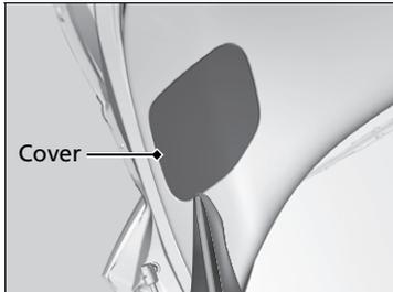
1. Remove the cover by prying on the edge of the cover using a flat-tip screwdriver.
