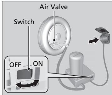
10. Turn on the air compressor and inflate the tyre to the specified air pressure.
