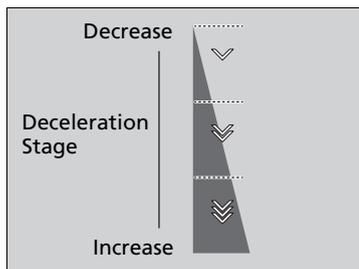
The default deceleration stage is . Each paddle selector operation makes a single stage deceleration change.
