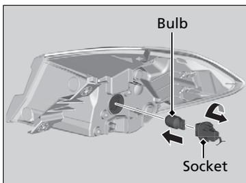
4. Turn the socket anticlockwise and remove it.
