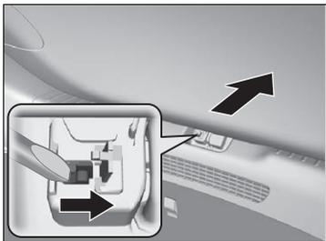
2. To open the tailgate, push the tailgate while sliding the lever to the right with the flat-tip screwdriver.
