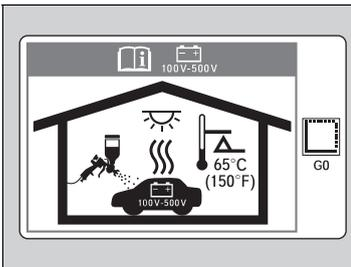
High temperature may damage the high-voltage battery used to power the electric motor.
