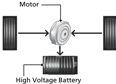
When decelerating without the accelerator being depressed or the brake pedal being applied, or while driving downhill, the electric motor acts as a generator that recovers a portion of the electrical energy that was used to accelerate the vehicle. This regenerative braking slows the vehicle in a manner similar to engine braking in a petrol-powered vehicle. You can control the rate of deceleration by using the deceleration paddle selector.
