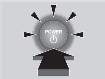
2. Depress the brake pedal and press the **POWER** button within 10 seconds after the beeper sounds and the **POWER** button changes from flashing to on.
