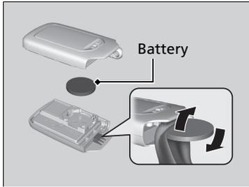
2. Remove the upper half of the cover by carefully prying on the edge with a coin.
