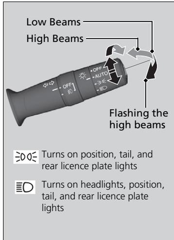
Rotating the light switch turns the lights on and off, regardless of the power mode setting.
