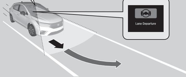
When you operate the turn signals to change lanes, the system is suspended, and resumes after the signals are off.
