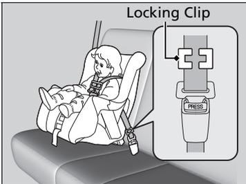
If your child restraint system does not come with a mechanism that secures the belt, install a locking clip on the seat belt.
