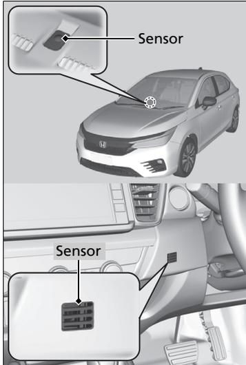
The automatic climate control system is equipped with sensors. Do not cover or spill any liquid on them.
