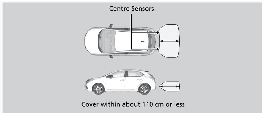
The system activates when the transmission is in **R**, and the vehicle speed is less than 8 km/h.
