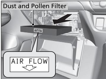
5. Remove the filter from the case.
