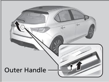
When all the doors are unlocked, the tailgate is unlocked. Press the tailgate outer handle and lift open the tailgate.
