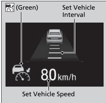
When ACC starts operating, the vehicle icon, interval bars and set speed appear on the gauge.
