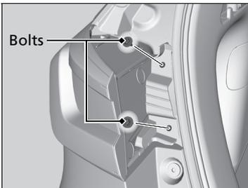
2. Use a Phillips-head screwdriver or socket to remove the bolts.
