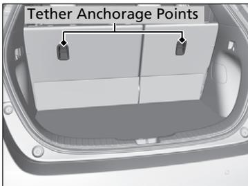
A tether anchorage point is provided behind each rear outer seating position. If you have a child restraint system that comes with a tether but can be installed with a seat belt, the tether may be used for additional security.
