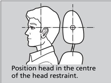
Head restraints are most effective for protection against whiplash and other rear-impact crash injuries when the centre of the back of the occupant's head rests against the centre of the restraint. The tops of the occupant's ears should be level with the centre height of the restraint.
