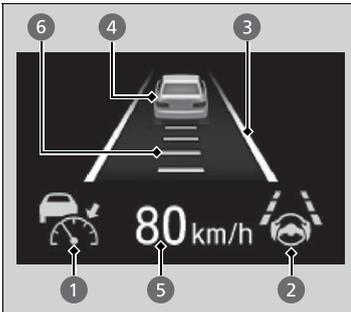
You can see the current state of Adaptive Cruise Control (ACC) and Lane Keeping Assist System (LKAS).
