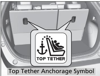
2. Place the child restraint system on the vehicle seat, then attach the child restraint system to the lower anchorages according to the instructions that came with the child restraint system.
