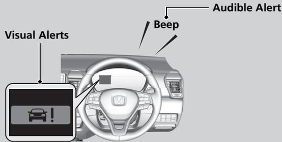
You can change the distance (**Far/Normal/Near**) between vehicles at which the system's earliest collision alert will come on through driver information interface setting options.
