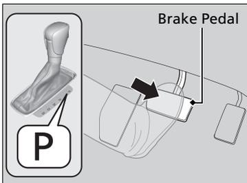
2. Check that the transmission is in **P**, then depress the brake pedal.
