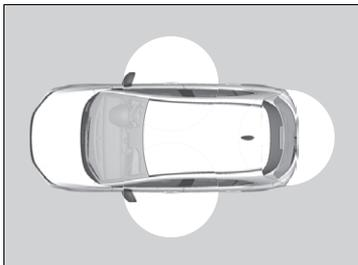
When you carry the keyless remote, you can lock/unlock the doors and open the tailgate.
