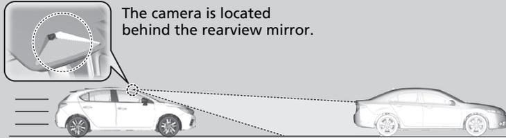
The system starts monitoring the roadway ahead when your vehicle speed is about 5 km/h or above and will search for a vehicle, pedestrian, or moving bicycle in front of you.
