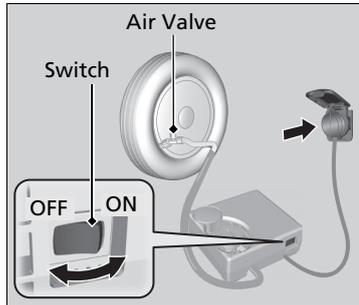
7. Turn the air compressor switch on to inflate the tyre.
